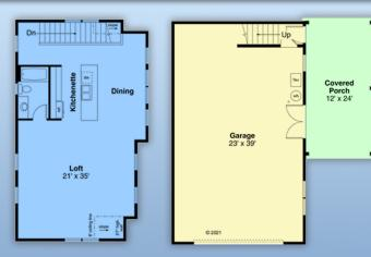
Garage Apartment Plan w/loft Dimensions: 36' wide x 40' deep Garage door: 16' wide x 8' tall 1 kitchenette + 1 full bathroom total under roof: 1836 square feet loft living area: 876 square feet garage area: 903 square feet stairwell: 57 square feet
